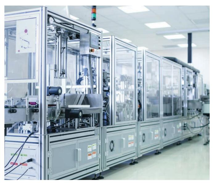
Marlon's excellent impact resistance and optical clarity combine to make it an ideal choice for safety and security applications. Easy to fabricate, it can be cut, bent or thermoformed into whatever shape is required to protect people or property.
